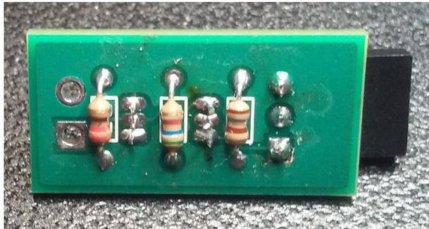
The resistors are shown soldered on the bottom, users can solder these on top as long as the layout is the same.
